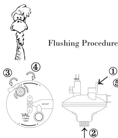
If you have the Floor Flushing Kit (VF200) all you have to do is Twist-n-Flush at the regulator (follow #2 - 5).
