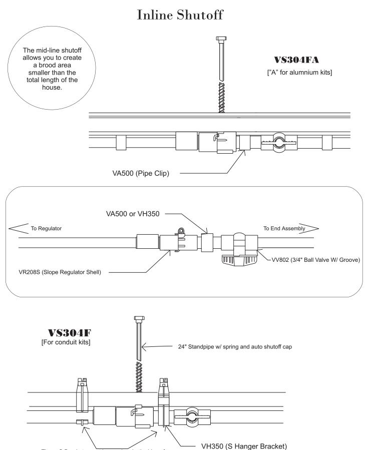
These S Brackets must be used on both sides of the regulator shell to keep the standpipe straight.
